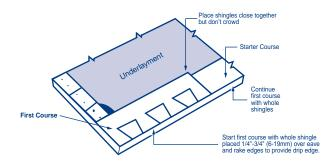
Trim 11" (279mm) from the first shingle in the course; then continue with full shingles across the roof. Strike a chalk line about every 6 courses to check parallel alignment with eaves. NOTE: Shingles may be laid from either left or right-hand side.
