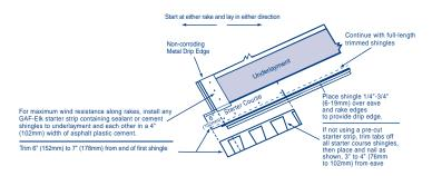
Start and continue second course as shown. Trim 6" (152mm) from the end of the shingle. Position the shingles in the second and subsequent courses flush with the tops of the wide cut-outs. This results in a 5-5/8" (143mm) exposure. Continue with full width shingles across the roof.
