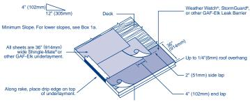
Along eave, put underlayment on top of metal drip edge.
