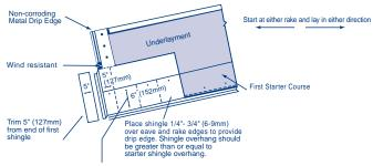
Minimum 1 nail per tab, 6" (152mm) up from butt end of shingle
