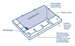
Trim 12" (305mm) from the first shingle in the course; then continue with full shingles across the roof. Strike a chalk line about every 6 courses to check parallel alignment with eaves. NOTE: Shingles may be laid from either left or right-hand side.
